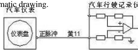
Figure 5-3 Installation the sensor vehicle speed signal wiring schematic drawing
